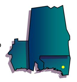
➤ With Smith #3 offline, multiple contingencies result in thermal overloads in the Panama City area, including the loss of Sinai Cemetery – Smith 230 kV T.L., which causes the Callaway - Gaskin 115 kV T.L. to become overloaded.
